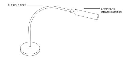
To set the light at different positions - bend any part of the "FLEXIBLE NECK" to move it. Never apply force to the "LAMP HEAD" to redirect the light. The "LAMP HEAD" can be gently adjusted downward from the "standard position" by 90 degrees and side-to-side by 270 degrees.
