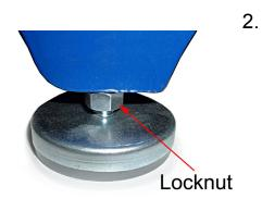
Set the machine in a flat area and level the pan by adjusting the legs (simply loosen the locknut, screw the leg in or out as required, and retighten the locknut).
